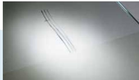
Guardian has conducted extensive testing that simulates the everyday abuse that glass receives—from coffee cups to key chains to cutlery. These test results measure and quantify the superior durability of DiamondGuard glass. The photo above shows the results of a scratch test, with regular glass at the top and DiamondGuard glass on the bottom.
